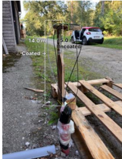
Figure 2. Experimental setup in National Park Bosland, Belgium (51.1623° N, 5.3169° E); both the Coated and Uncoated regions are in the indicated while rectangle; the white is coated with aluminum spray, and the black remains the original.
