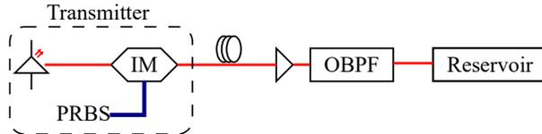
Figure 1: Schematic representation of the simulation setup to generate data for the signal equalization task. The input pseudo-random bit sequence (PRBS) signal is modulated onto a laser signal, transmitted over a fiber link, amplified and filtered, after which the field of the optical signal is saved to file to be used as input to the photonic reservoir simulation model. OBPF - Optical band pass filter.
