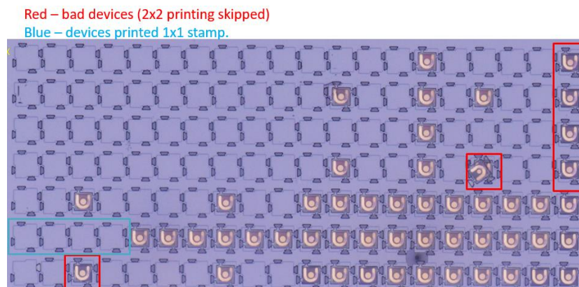
Fig. 5. Top view of the source wafer after completing the transfer printing. Collapsed or broken devices are shown in red which were skipped by the 2x2 array stamp. The blue rectangle indicates devices that were picked and printed in 1x1 mode.
