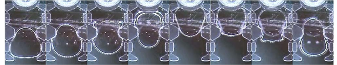
Figure 7: Captured frames of the HPC droplet motion in the microfluidic optical switch with TPS as the ambient liquid.
