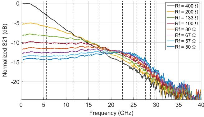
Fig. 3. Measured S21 of the coherent receiver with TIA for different transimpedance settings, i.e.  $R_f = 400 \Omega/N$  with  $N = 1, 2, \dots, 8$ , normalized to the low frequency gain at the largest  $R_f$  setting. The dotted vertical lines indicate the 3-dB bandwidth corresponding to the decreasing  $R_f$  values.
