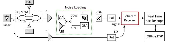
Fig. 2. Schematic of the characterization setup of the QPSK/16-QAM coherent receiver.
