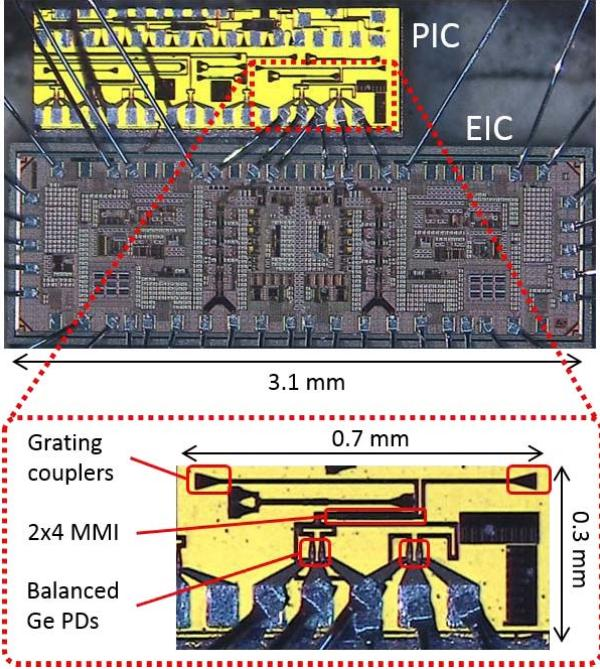
Fig. 1. Micrograph of the photonic integrated circuit (PIC) wirebonded to the electronic integrated circuit (EIC) together with a more detailed view of the PIC-layout. The PIC was kept larger than the dimensions of the coherent receiver for ease of dicing and assembly.
