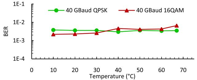
Fig. 5. Temperature dependence of coherent receiver in terms of BER for a fixed OSNR (corresponding to a BER of  $\sim 3 \times 10^{-3}$  at room temperature) for 40 GBaud QPSK (green) and 16-QAM (red).
