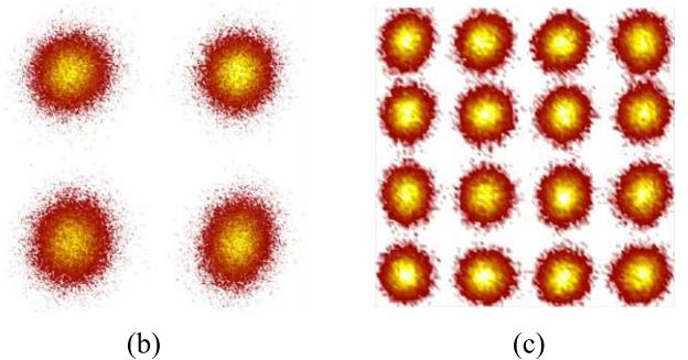
Fig. 4. (a) Measured BER versus OSNR (0.1 nm bandwidth). QPSK is shown as green and 16-QAM as red, 28 GBaud curves are dotted, 40 GBaud curves are full; Received constellations for (b) 80 Gb/s QPSK with  $20 \text{ dB}$  OSNR and (c) 160 Gb/s 16-QAM with  $30 \text{ dB}$  OSNR.
