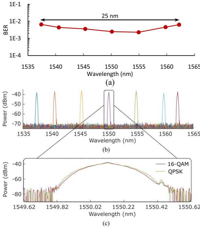
Fig. 6. (a) Wavelength dependence of the coherent receiver in the C-band in terms of BER measured over a range of  $1550 \text{ nm} \pm 12.5 \text{ nm}$  for 40 GBaud 16-QAM. (b) Optical spectra for each investigated channel. (c) Detailed example of an optical spectra for a carrier at 1550.12 nm.
