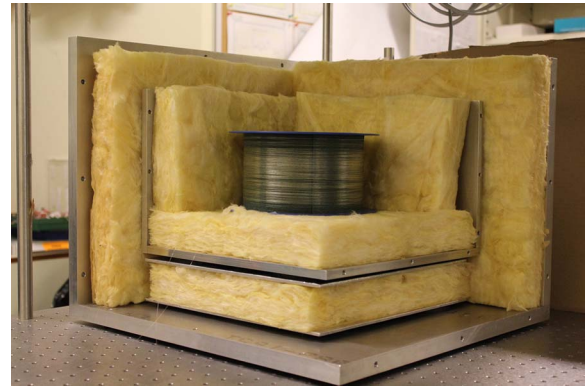
Fig. 4. Isolation system of the delay loop, open. It consists of two aluminum boxes: a small box made of 1 cm thick plates inside a bigger box made of 2 cm thick plates. The inner plates of both boxes are covered with stone wool. Each box is isolated from the base on which it rests by sorbothane sheets that absorb vibrations.
