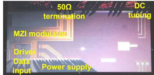
Fig. 4. Annotated optical microscope image of the frontend integrated BiCMOS driver and carrier depletion modulator during testing.
