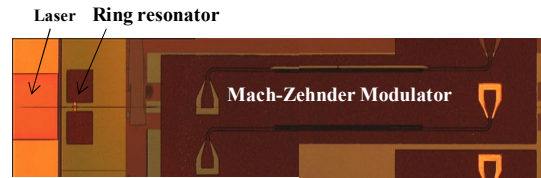
Fig. 5. Optical microscope image of the III-V source and carrier depletion modulator integration.
