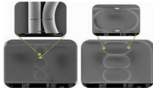
Figure 4. SEM images of 3 rd order MRR and race-track resonators for single- and multi- \lambda AOWC
