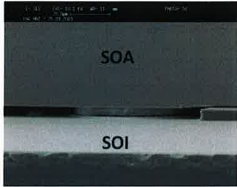
Figure 4: SEM image demonstrating the SOA flip-chip bonded in the SOI board
