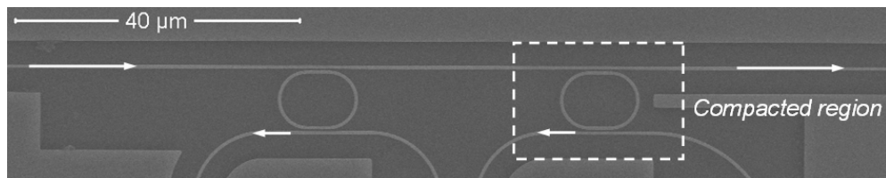
Fig. 1. Overview of the experiment: the right ring is trimmed by electron beam compaction; the left one is kept original as a reference to exclude temperature or ambient variations.
