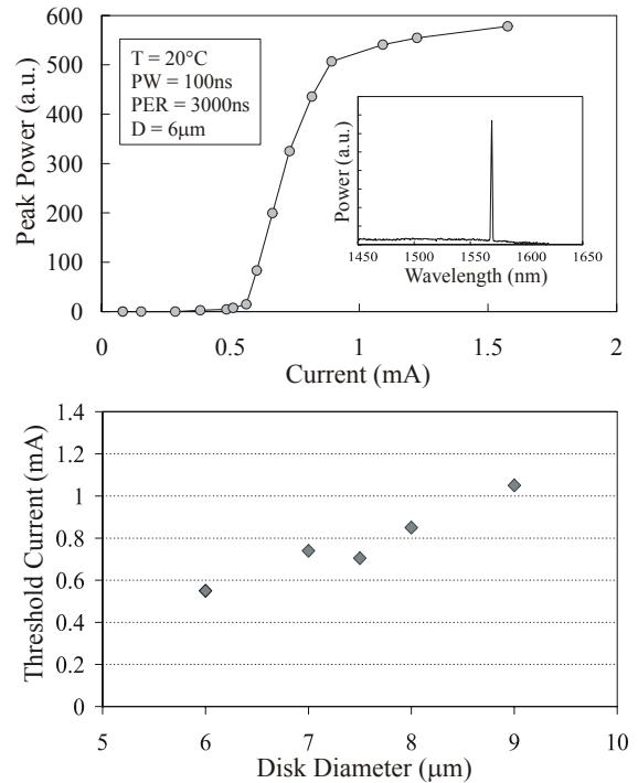
Fig. 2. Top: Light output vs. current for a disk diameter of 6 $\mu\text{m}$ . Inset: lasing spectrum for 0.75mA. Below: threshold current vs. disk diameter.
