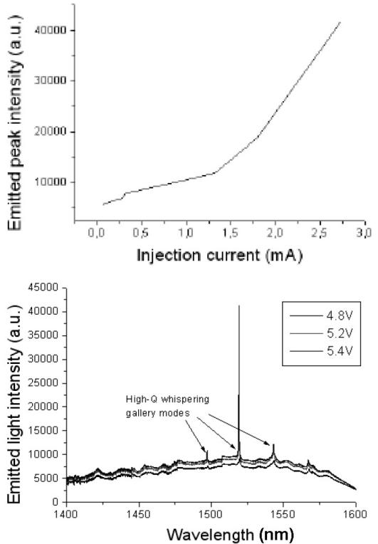
**Figure 3** PI-curve and emission spectrum of a membrane microdisk laser (diameter= $8\mu\text{m}$ )
