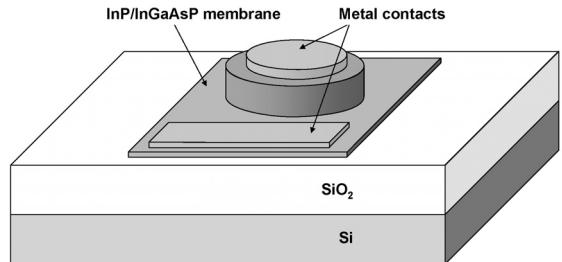
Figure 1. General layout of the membrane microdisk laser
