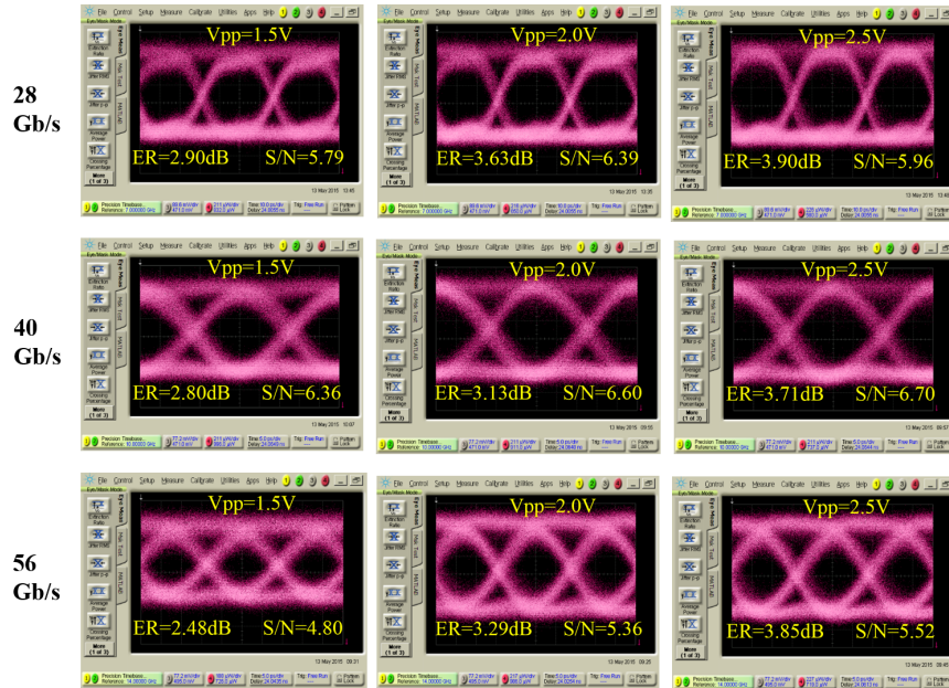
Figure 6.20: Measured eye diagrams from Ge EAM, at room temperature, at 1610 nm with 1.5 V pp , 2.0 V pp and 2.5 V pp voltage swing and with data rates of 28 Gb/s, 40 Gb/s and 56 Gb/s with input power of 0 dBm before the modulator in the device.
