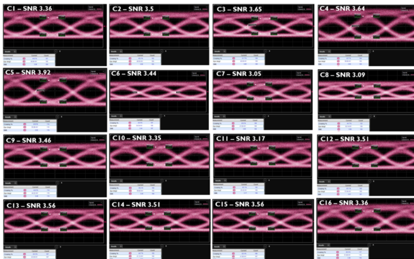
Figure 6.24: 56 Gb/s PRBS eye diagrams at 1565 nm for 16 channel GeSi PD, each 60 \mu\text{m} long, and operated at -2 V [14].
