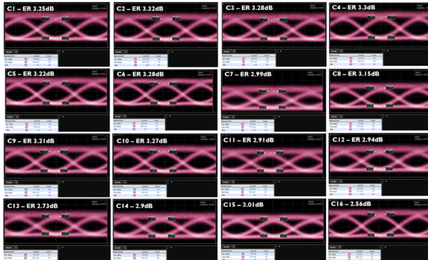
Figure 6.23: 56 Gb/s PRBS eye diagrams at 1565 nm for 16 channel GeSi EAM, each 40 \mu\text{m} long, and driven with 2.5 Vpp voltage swing [14].
