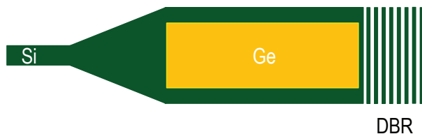
Figure 5.1: Improving the responsivity at long wavelength using a DBR following the Ge waveguide.
